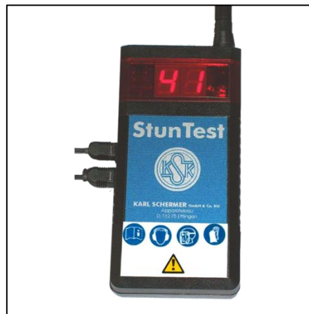
Fig.5-29 Display of the muzzle velocity
