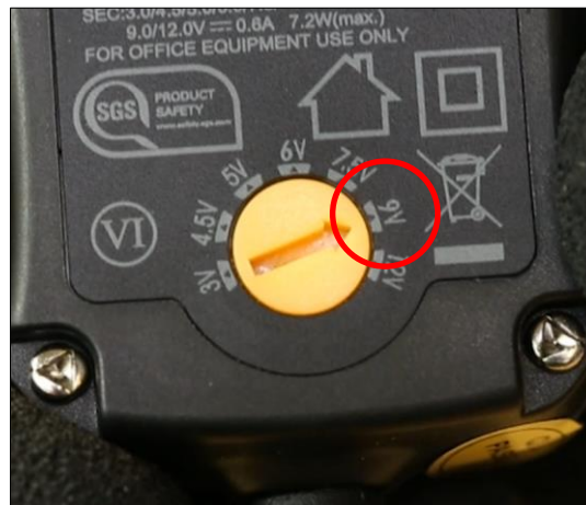
Fig.5-22 Adjusting the power supply
