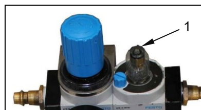
Fig. 5-2 Filling the service unit
