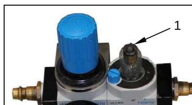
Fig. 5-2 Filling the service unit
