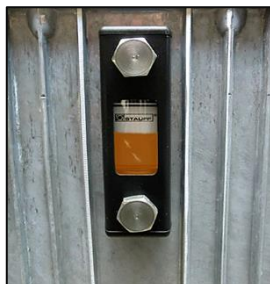
Fig. 8-1 Optimum oil level
