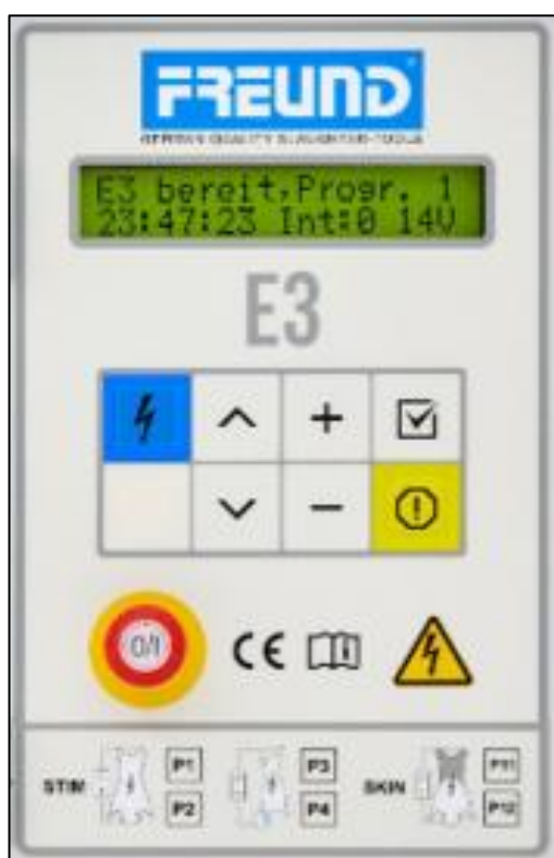
Fig. 3-13 Display and operating elements STIM-E3
