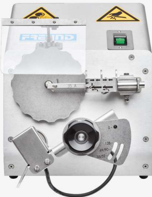
*Figure: Standard variant with steeling device for blades Ø 35-52 mm
